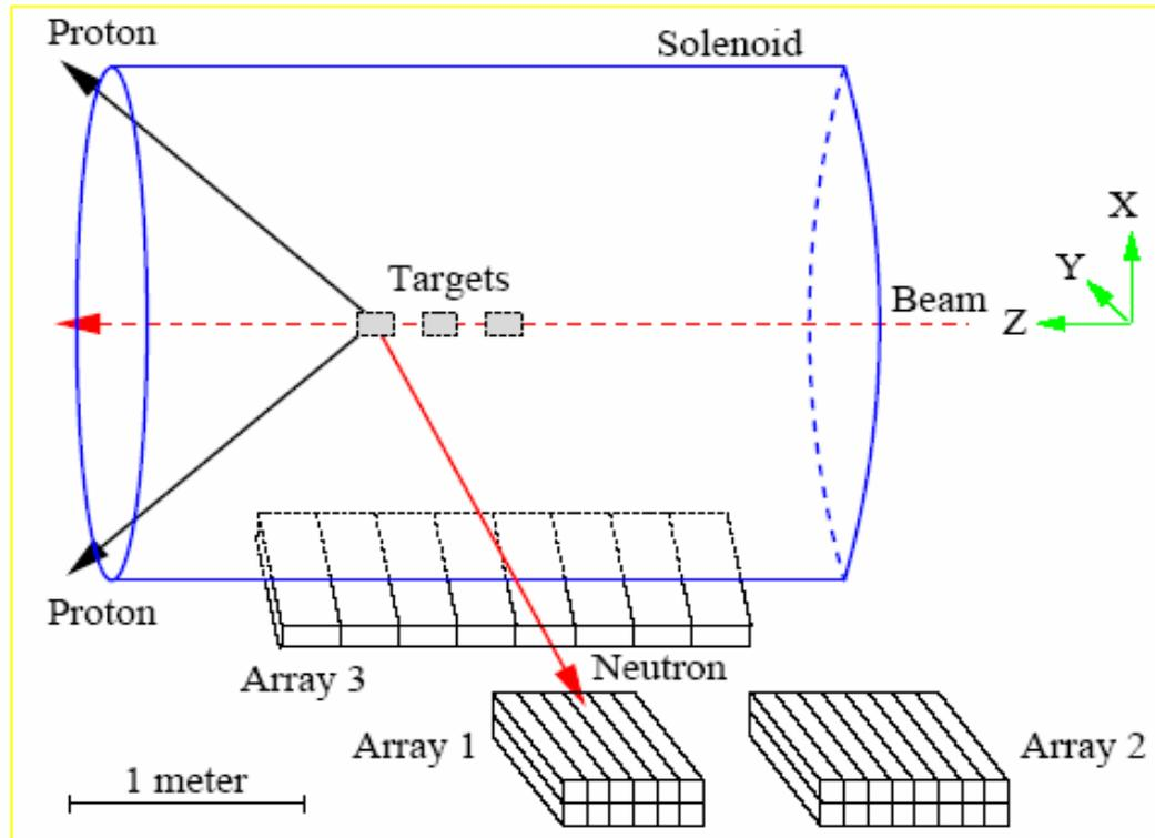
Figure I.3: A schematic view of the EVA solenoid and the neutron counters in the 1998 measurement.
